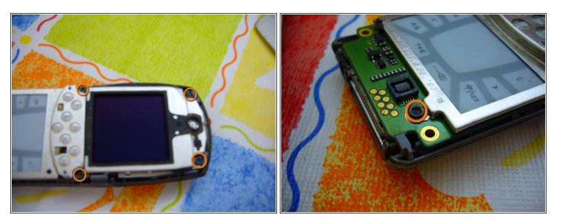
• Remove 5 trox screws that are holding the screen and the touch pad.
