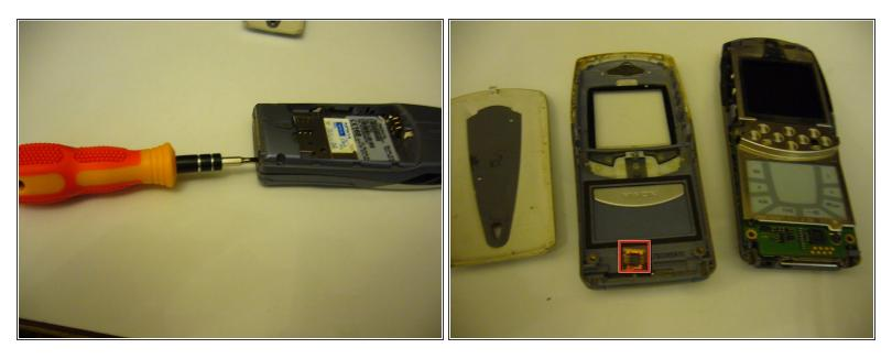
Remove the front panel by pulling it or using an
