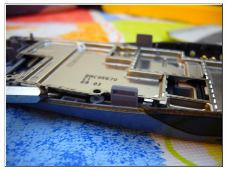
• Removing the EMI shield.Pry around the edge of the shield to remove it.
