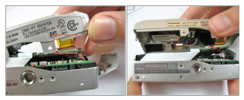
A Be careful not to damage the ribbon cable when opening. Ensure it is still attached.
