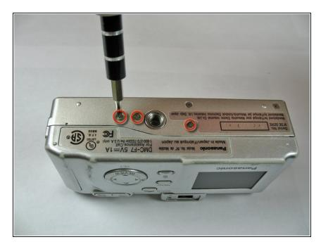
• Use the Phillips #00 screwdriver to remove the three 2.8 mm screws on the bottom of the camera.
