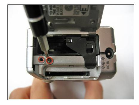
Using the Phillips #00 screwdriver, remove the two 2.8 mm screws located under the hatch.
