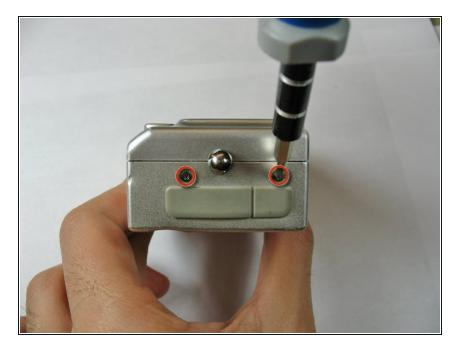
• Use the Phillips #00 screwdriver to remove the two 2.8 mm screws on the side of the camera.
