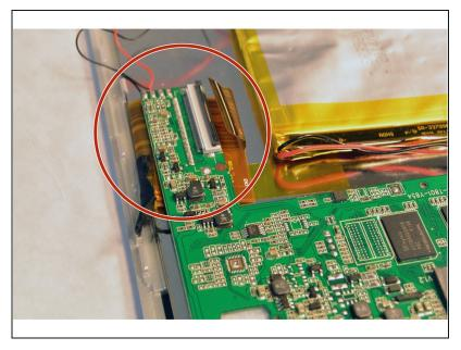
Disconnect the other ZIF connector on the opposite side of the motherboard.
