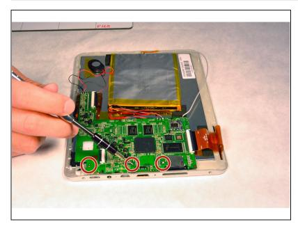
• Using the Phillips #1 screwdriver, remove the three screws from the motherboard..
