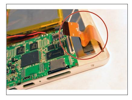
• Open the ZIF connector. Then, remove the ribbon that connects the motherboard and the screen.
