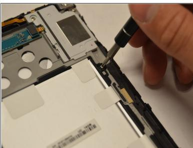
Remove the six 4 mm Phillips #00 screws that hold the battery in place.
