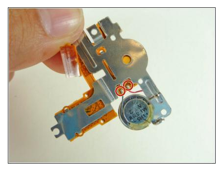
Desolder the speaker at the two solder points and reattach the new speaker.
