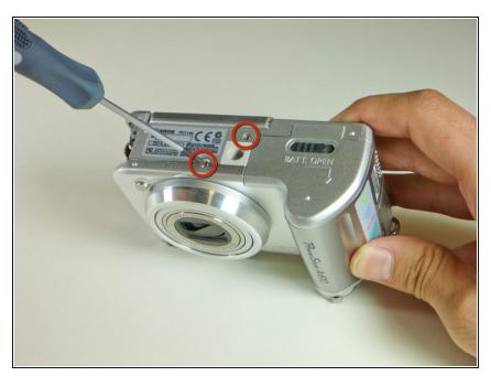
Remove the two screws on the bottom panel of the camera.
