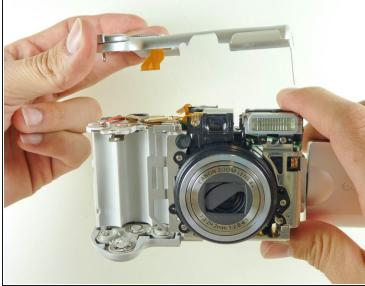
Using an opening tool, push the black attachment away from the white connection piece to detach the connector ribbon.
