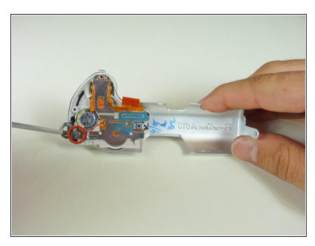
Remove the 3 mm screw holding the metal frame.
