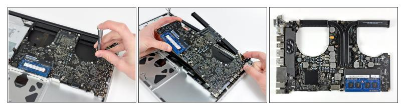
• The main board lifts out along with the heat sink still attached. This is a nice feature, as this way you have to remove the heat sink and reapply thermal paste only if you're completely replacing the logic board.
