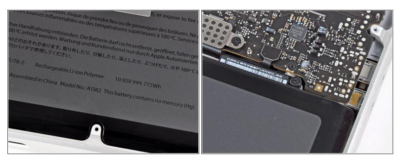
This machine boasts a 77.5 Watt-hour battery. That's the same capacity as the previous revision, but the reported battery life has gone from 8-9 hours to 7 hours. Has performance really decreased, or is Apple being more realistic with their estimates? We don't have 7 hours to wait and find out, so we'll have to leave that investigation to someone with a fully-assembled unit.
