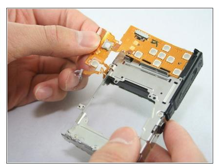
By hand, gently unfold the function button board and lift it off the frame.
