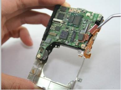
• Gently pull straight out on the ribbon to disconnect it from the logic board.
