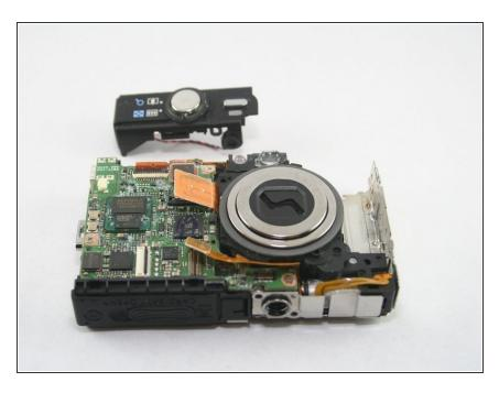
The shutter button assembly should now be removed.
