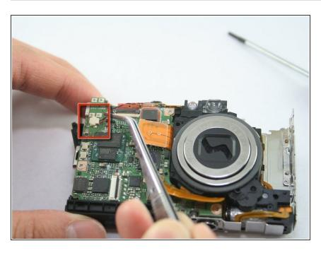
Use the tweezers to disconnect the microphone cable.
