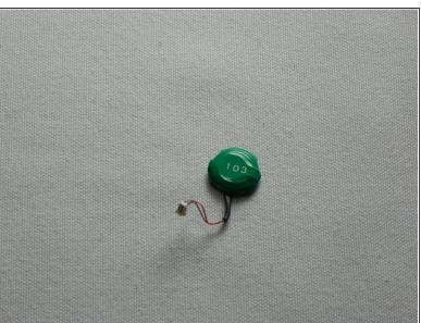
once the joypad key have been removed use the tweezers to carefully maneuver the wire out of its clip releasing the battery
