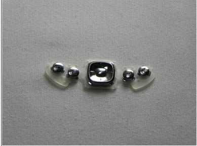
Once removed you can easily separate the keys from the body.
