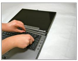
Use a spudger to partially lift the hinge cover.
