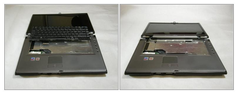
After the ribbon has been detached, carefully remove the keyboard.
