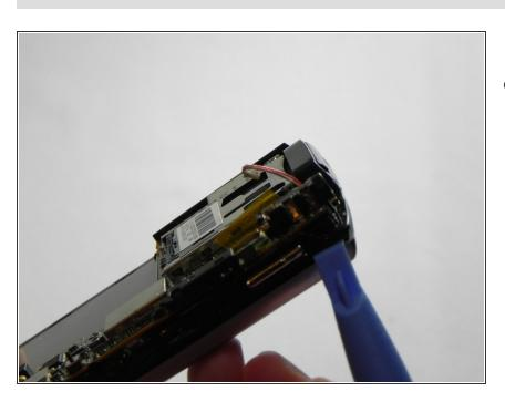
Next, use a plastic removal tool and separate the silver front case from the black frame. To reassemble your device, follow these instructions in reverse order.
