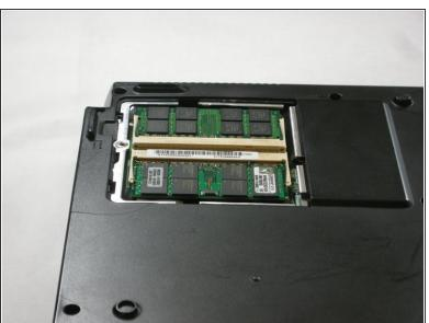
Remove the RAM cover by lifting it with your finger.
