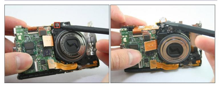
• Use spudger to carefully lift the LED light off the upper-left corner of the lens.
