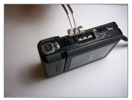
Remove the three combined buttons so they are not misplaced.
