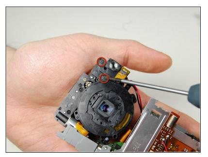
On the backside of the camera where the indicator lamp is located, remove the two screws with a screwdriver
