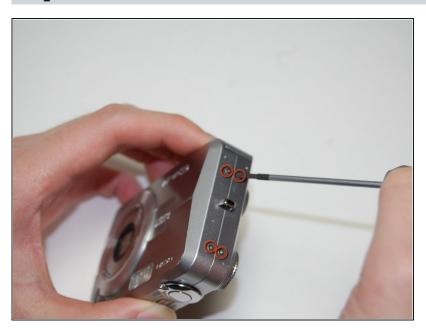
With the screwdriver, remove the four screws on the side of the speaker.
