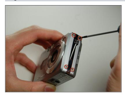
• Remove the four screws on the side with the screwdriver.
