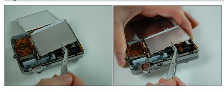
• With tweezers, pry off the LCD casing which is taped on to the frame.
