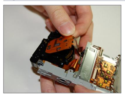
Remove the large orange ribbon previously held in by screws from the camera and set it asside.
