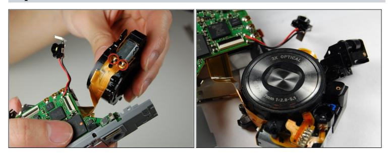
• The lens is now detached from the camera except for the ribbon soldered onto the logic board.
