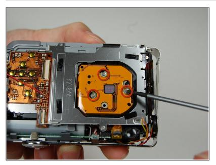
On the back of the camera where the LCD screen was, remove the 3 screws located behind the lens.
