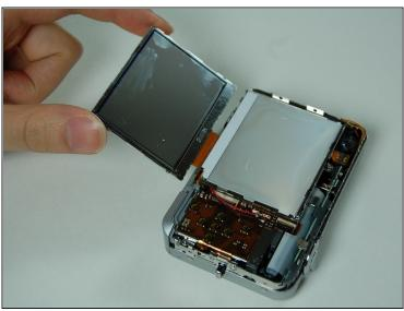
• Use tweezers to lift up the LCD screen away from the camera.
