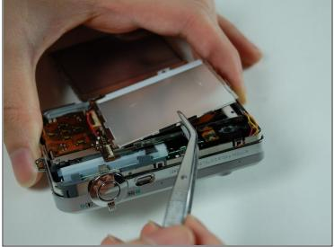
• Use tweezers to slowly pry off LCD casing by lifting and moving it off the camera.
