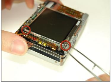
• Use tweezers to pry the LCD screen off from the opening.
