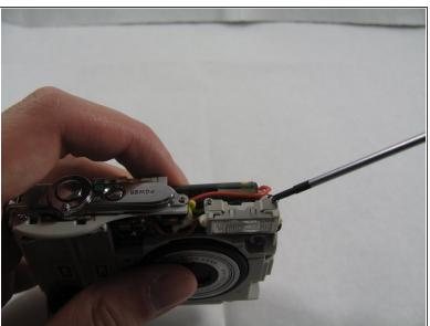
Remove the two 2.7 mm screws using a #00 screwdriver.
