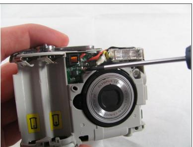
Remove the 2.7 mm screw holding the front circuit board in place.
