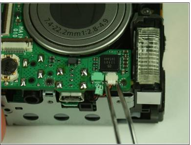
Detach the white-capped and green-capped wires, which sit near the flash.
