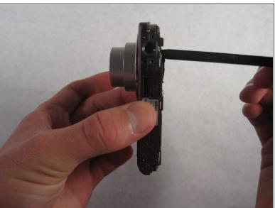
Place the spudger on the outermost surface of the lens and push in. This will extend your camera lens.
