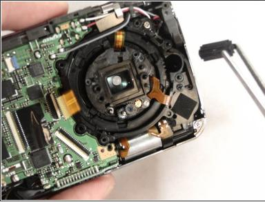
Using tweezers, remove the cylindrical gear from the camera.
