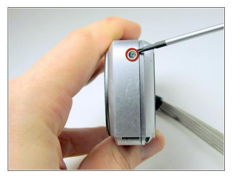
Locate the 5.3mm silver screw on the edge closest to the upper left corner of the LCD screen and remove it.
