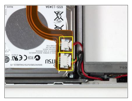
Disconnect the IR and sleep light cables from their connectors above the hard drive.
