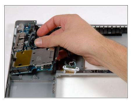
Lift the left I/O board up from the right side and slide it out of the computer.
