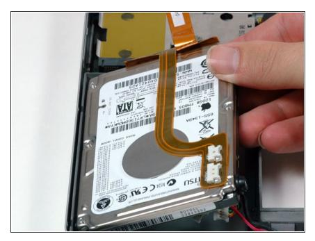
Lift the hard drive up from the right side and remove it and the attached cable from the computer.
