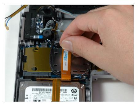
Peel up the orange hard drive cable from above the ExpressCard cage.
