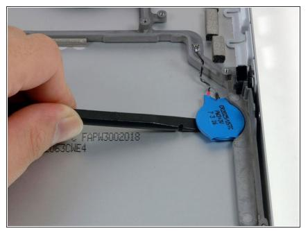
Use a spudger to pry up the PRAM battery off the lower case.
