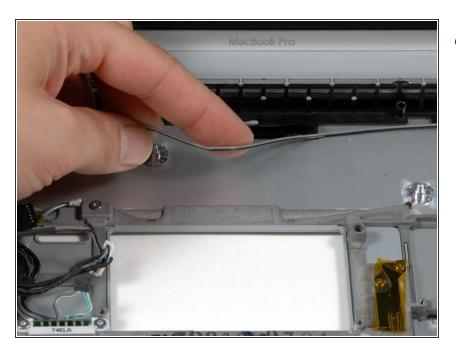
Continue to free the speaker cable from the black tape until it is free from all three sections of tape.
