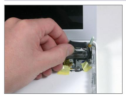
• Lift the right speaker out of its housing and set it to the side.
