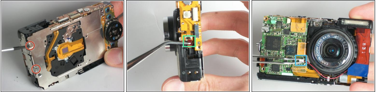
**⚠ Use caution when removing the flash, as the capacitor may still have a charge.**
