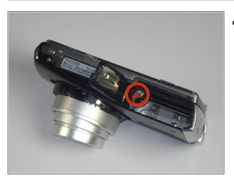
Remove the battery by pushing the red lever to the side.
