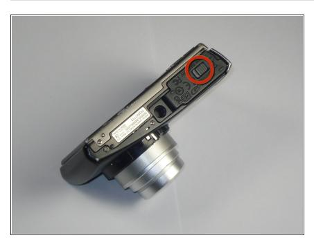
Using your thumb, slide the gray button to open the battery compartment.
