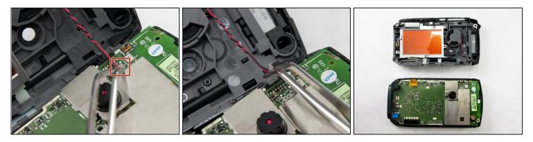
• Using tweezers, squeeze the plastic head of the black and red wound wire cable. This will detach the cable from the circuit board and fully separate the two halves.
