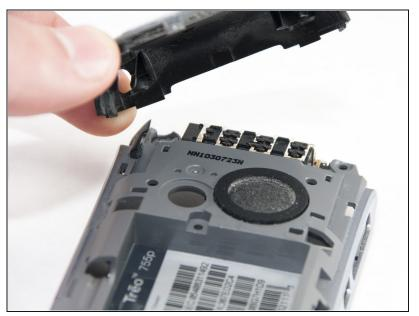
• Lift off the top of the back cover from the phone frame.
