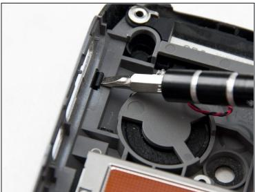
Press in the four black clips using a spudger to pop off the upper-back cover.
