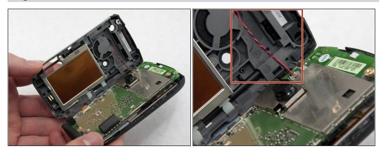
• Slowly unfold the back casing away from the front casing revealing the red and black wound wire speaker cable, marked by the red box.
