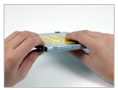
Rotate the drive and disconnect the orange ribbon cable from the optical drive.
