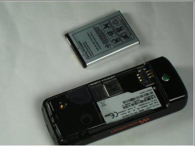
Pop the battery out of its slot by lifting it up.
