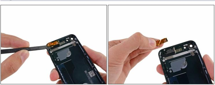
Use the flat end of a spudger to gently pry the antenna up from its foam adhesive backing.
