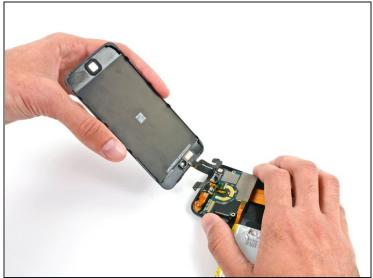
Remove the display assembly from the iPod.
