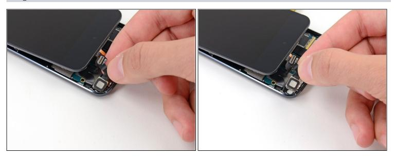
• Lift the rear-facing camera up out of its socket and remove it from the iPod Touch.
