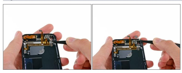
• Use tweezers to remove the small metal backing plate from the power switch section of the button ribbon cable.
