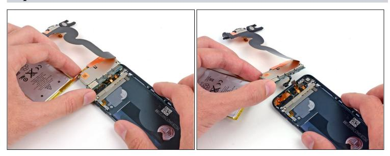
• Remove the logic board assembly from the rear case of the iPod.
