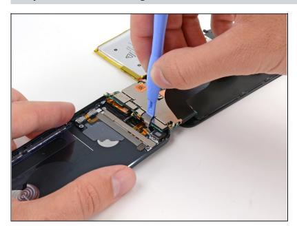
Use the edge of a plastic opening tool to disconnect the rear-facing camera ribbon cable from the back of the logic board.
