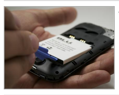
Using a plastic opening tool or finger, pull out the battery.
