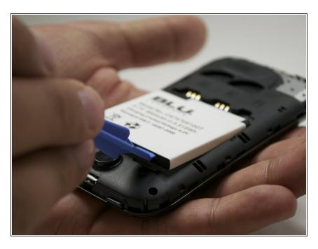
Using a plastic opening tool or finger, pull out the battery.
