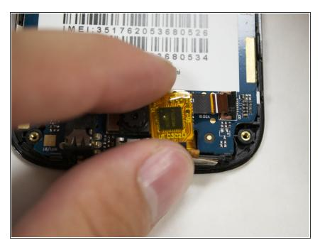
Pull the ribbon cable out of the ZIF connector.
