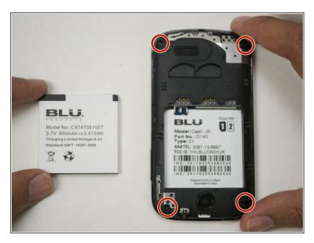
Remove the four 4.0mm Phillips #1 screws.
