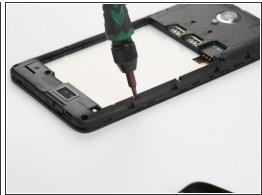
• The GPS, wifi, Bluetooth integrated antenna is located at top left. On the right side, there is one of the two network antenna, the other network antenna is located at the bottom of the phone. SIM cards slots and TF card slot are under the camera.
