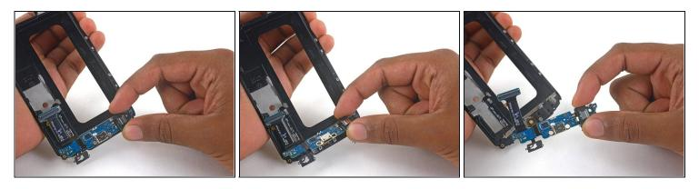
*i* Flip the frame over again and lift up the daughterboard to peel it off the display frame.
