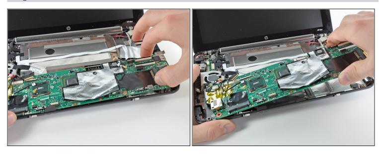
• Carefully lift the motherboard from its right edge and remove it from the lower case, minding any cables that may get caught.
