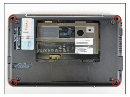
Remove the four 7 mm Phillips screws that secure the upper case to the lower case.
