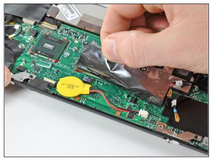
i If present, carefully peel back the piece of black film attached to the heat sink to reveal the PRAM battery and its cable.
