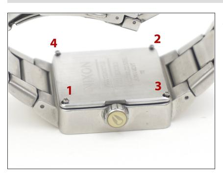
Tighten screws in a star pattern until the backplate is tight.
