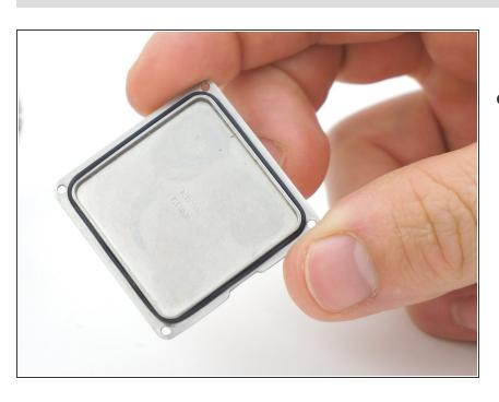
Seat the gasket back onto the back plate.
