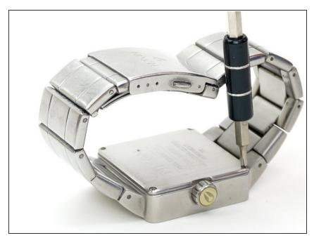
On a flat surface, use the PH00 screwdriver to remove the four screws from each corner, and set them in a safe place.
