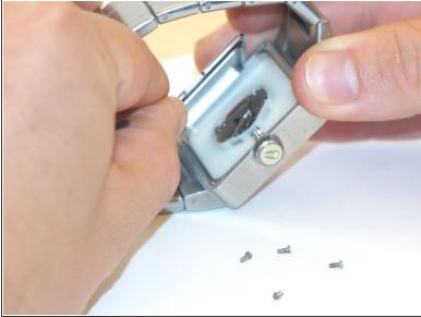
• Gently lift the back plate, and be careful to not damage the rubber gasket.
