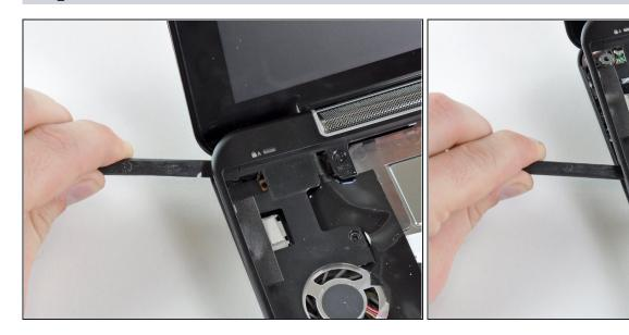
• Repeat the same procedure as mentioned in the previous step to release the clips along the left side of the upper case.
