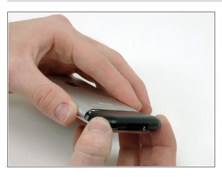
Grasp the antenna cover on either side and slide it up and away from the iPhone. This requires some force. If it does not come free, ensure that the antenna cover is lifted up enough to free the catches.
