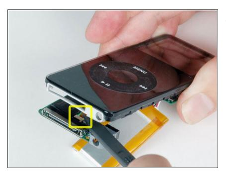
Use a spudger to slide the click wheel ribbon out of its connector.
