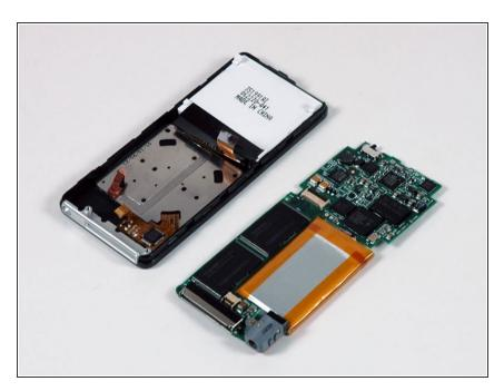
The logic board and battery are now free from the iPod.
