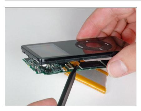
Use a spudger to slide the display ribbon out of its connector.
