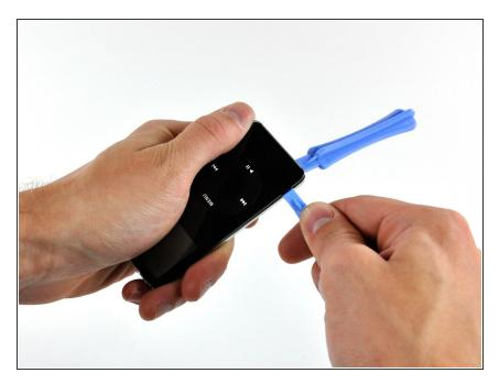
Insert a small iPod opening tool into the seam on the Hold button side of the iPod, with the edge of the tool pointing toward the rear panel.
