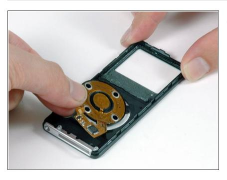
Lift the click wheel out of the front panel.
