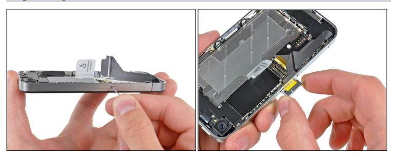
Use a SIM card eject tool or a paperclip to eject the SIM card and its holder.
