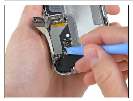
Use a plastic opening tool to pry the lower antenna connector up off its socket on the logic board.
