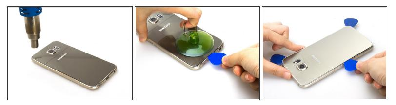
Remove the back cover at first. It's a pity that we only have a S6 with broken back cover to show how to do camera lens glass replacement.
