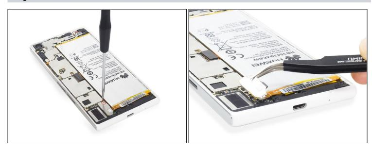
Remove battery securing bracket.
