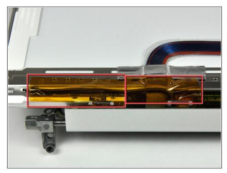
if necessary, remove the two pieces of tape covering the inverter leads.
