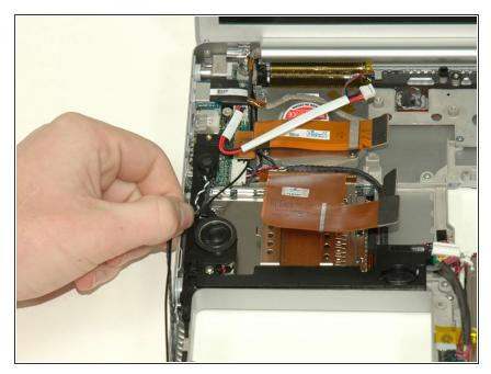
Deroute the Bluetooth and RJ-11 cables from around the left side of the speaker.
