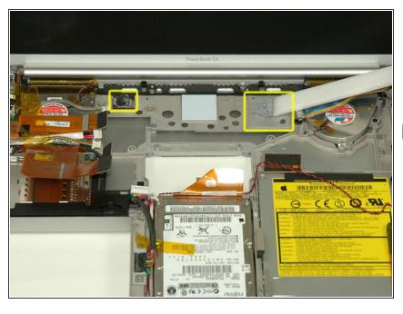
Important: when you reinstall a logic board, you'll need to replace the thermal paste that goes between the processor on the logic board and the heat sink. Failure to remove the old paste and apply a new layer can cause the computer to overheat and sustain damage.
