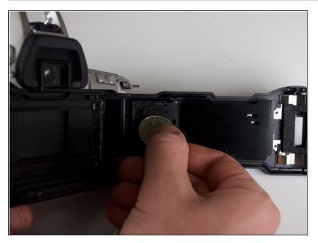
Use a coin to twist open the battery compartment (twist counterclockwise).
