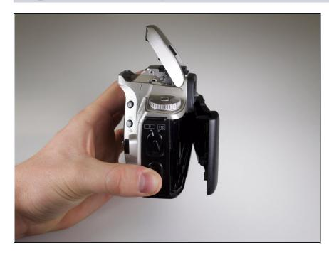
Press up firmly on the backcover release on the right side of the camera to release the back panel.
