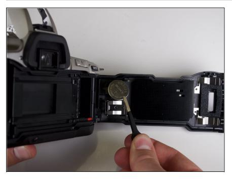
Use tweezers to take out the old clock battery and replace it with a new one.
