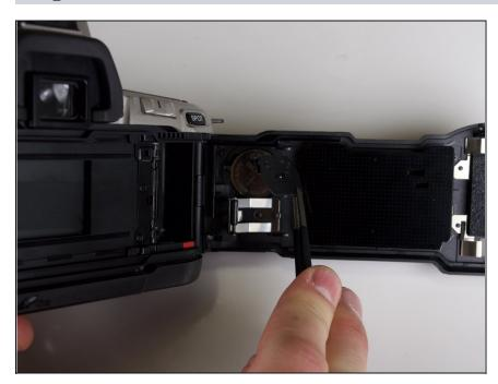
• Use <u>tweezers</u> to lift off the battery compartment cover.
