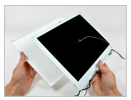
Lift the rear bezel off the display.
