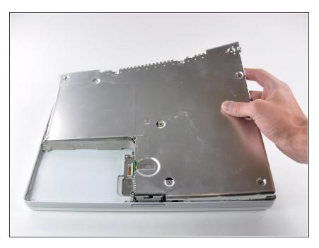
Lift the bottom shield off.
