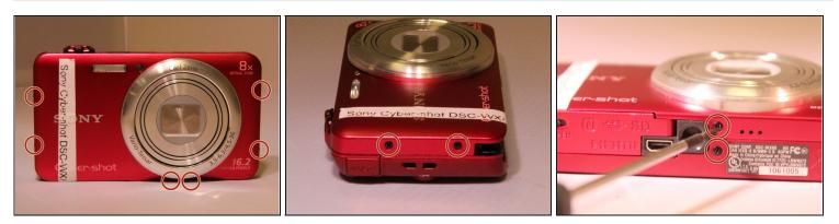
Remove all six #00 screws holding the outer chassis together with a Phillips #00 screwdriver.
