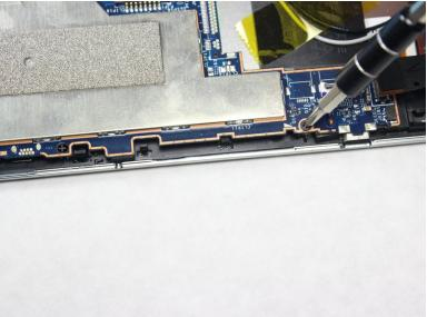
Remove the 4 1.6mm screws with a J0 head.
