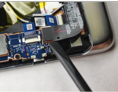
Locate the LCD cable connector and gently pry it directly up with a spudger.
