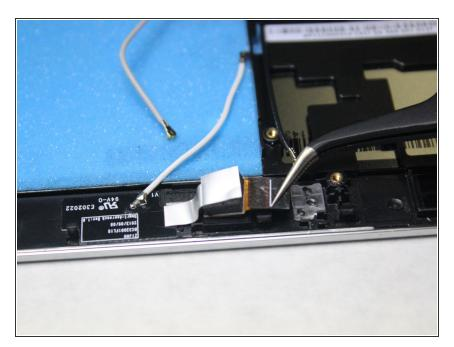
Disconnect the ribbon cable using the tweezers
