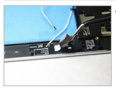
Lift the camera up with tweezers to remove it
