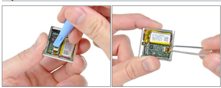
• Use the edge of an iPod opening tool to flip up the retaining flap on the control button cable ZIF socket.
