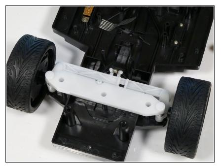
• Gently pull the steering column up and remove it along with the wheels
