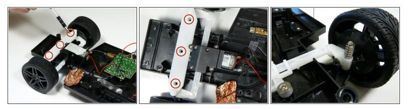
• Unscrew the three 2.5mm Phillips #00 screws from the white steering column.
