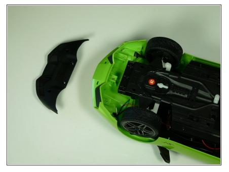
Lift the front part of the underbody and pull it out from the main underbody.
