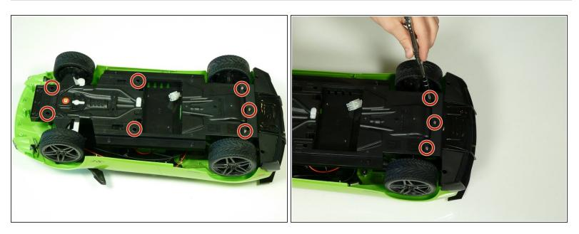
• Unscrew the remaining seven 9mm Phillips #00 screws from the underbody of the car.
