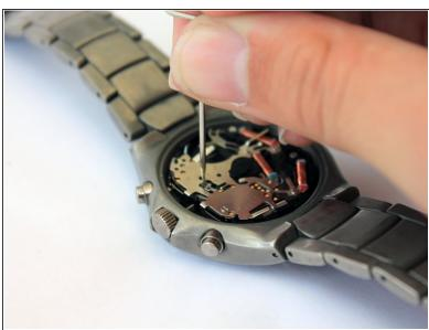
Press the release button for the Time Setting Dial using a thin pin.
